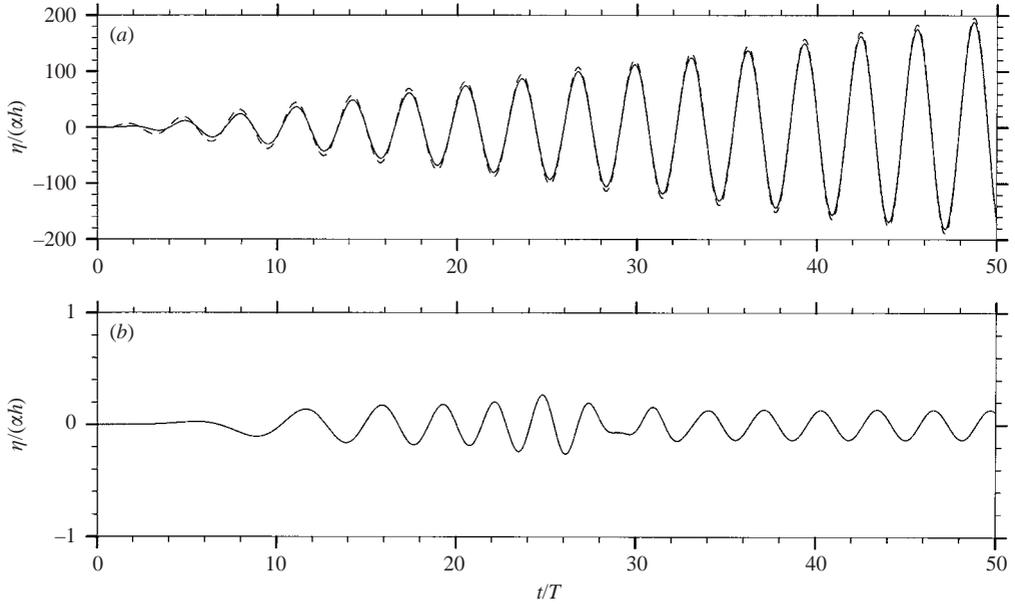
FIGURE 6. Free-surface elevation  $\eta$  as a function of time  $t$  for a trapping structure forced to oscillate at the trapped-mode frequency  $\omega_0$ : (a) mid-point, (b) far field. In (a) the numerical solution (—) is compared with the leading-order asymptotic solution (---) whilst (b) shows only the numerical solution.
