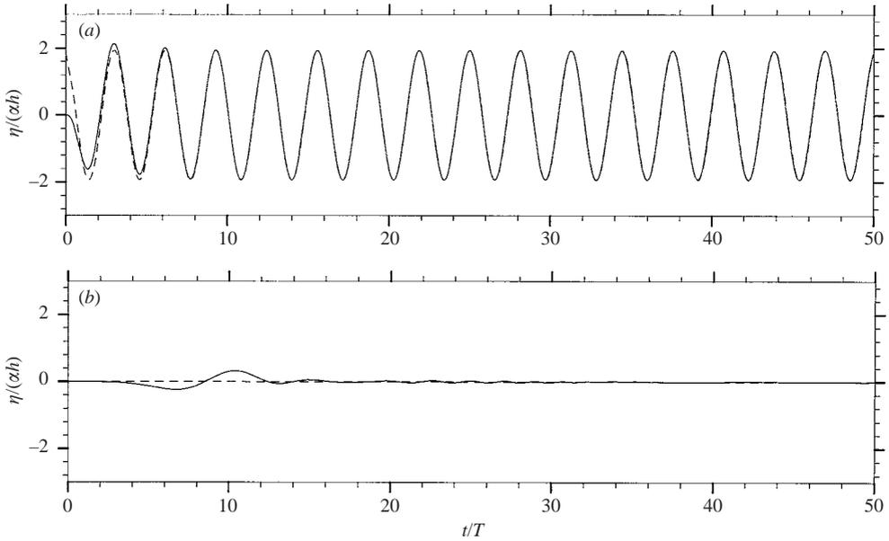
FIGURE 3. Free-surface elevation  $\eta$  as a function of time  $t$  for a trapping structure after a transient disturbance: (a) mid-point, (b) far field. The figures compare the numerical solution (—) with the asymptotic solution (---).
