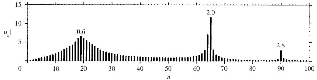
FIGURE 13. Discrete Fourier transform of the free-surface elevation shown in figure 11(a). Here  $|u_n|$  is  $N^{-1/2}$  times the amplitude of the Fourier component with index  $n$ , where  $N$  is the number of samples in the signal, and the numbers within the plot are the non-dimensional frequencies  $\Omega = \omega/\sqrt{g/h}$  corresponding to the peaks at  $n = 19, 65$  and  $90$ .
